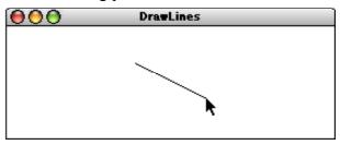
Because the original point and the mouse position appear to be joined by some elastic string, this technique is called *rubber-banding*.
